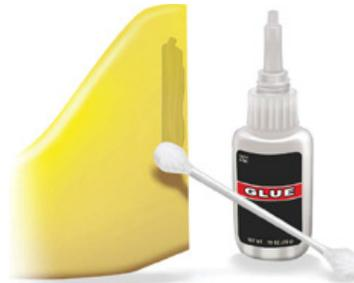
If you're having trouble getting your tape hinges to stick to your foam airplane, use a Q-tip to apply a thin coating of medium or thick foam-safe CA to the area where the tape will be applied. Let the adhesive air dry (don't use kicker!) and then apply the tape. The hinge material will stick more securely and will last much longer than if it were applied to the untreated foam surface.
