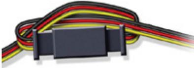
If one of your model's control servo connectors become unplugged during flight, at best, you're going to have a really tough time getting it back on the ground in one piece. At worst, you could lose the model completely due to a serious crash. By simply crossing your servo lead end like this and forming a half-knot at the connection, you can be sure the connectors won't come undone even while under extreme forces during aerobatic flight.
