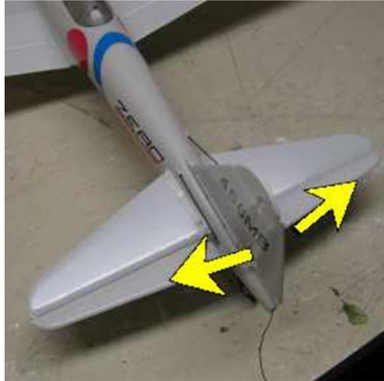
controls the Yaw of the airplane. left or right. This picture shows motions of the rudder will control
