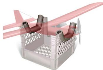
Using an old milk crate (readily available everywhere!) and some water pipe insulation foam, makes an inexpensive, yet very sturdy model airplane maintenance and support stand. It's also big enough to use as an equipment caddy to transport your battery charger and field equipment.
